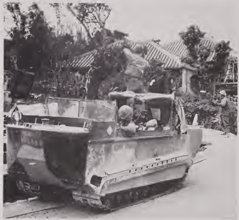
FIGURE 78. United States Marines on Okinawa string telephone wire with aid of M-29C Weasel.
